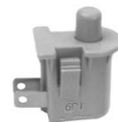
Order No. 31 - 9664 Plunger Interlock switch replaces Exmark 1-740275. Single post, right angle snap in mounted. Normally closed.
