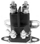
Order No. 31 - 10772 Universal starter solenoid 4 pole, 12 volt. Terminal post will accommodate both 5/16" & 1/4" terminal connectors, Mounting bracket will accommodate both chassis and wall mount configurations. Replaces Exmark 1-513075.
